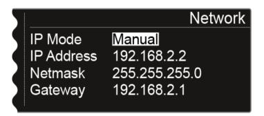
Press the jog dial to switch between the individual network configuration items.
