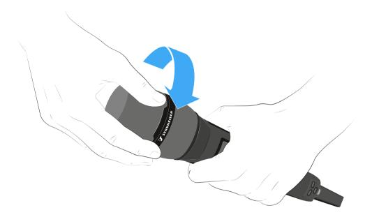
**i** With some microphone modules, the upper part of the microphone basket can be screwed off. Ensure that you always completely unscrew the microphone module.
