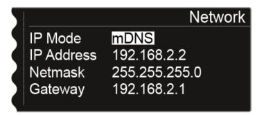
• IP Mode Manual: You can manually set the IP address, netmask, and gateway.
