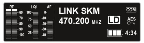
In the displays, the home screens for both channels display the **channel-specific status information** such as the reception quality, battery life, audio level, and so on. See Home screen.
