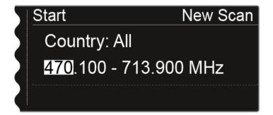
You can adjust the value by turning the jog dial. Press the jog dial to move back and forth between the individual points of the frequencies.
