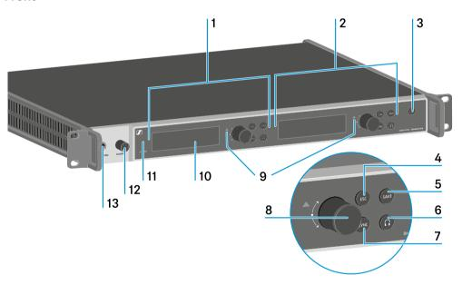
1 Displaying and using channel 1 (CH 1)
