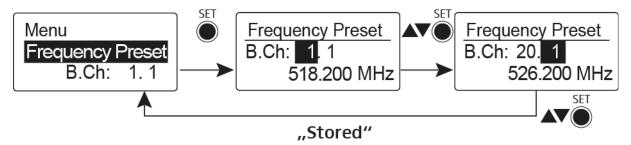
While you work in the Frequency Preset menu, the RF signal is deactivated.
