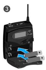
▶ Close the battery compartment.The cover locks into place with an audible click.
