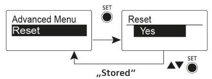
When you reset the plug-on transmitter, only the selected settings of the pilot tone and the  ${\bf U}$  frequency bank are retained.
