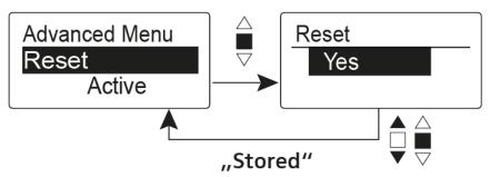
When you reset the wireless microphone, only the selected settings of the pilot tone and the  ${\bf U}$  frequency bank are retained.
