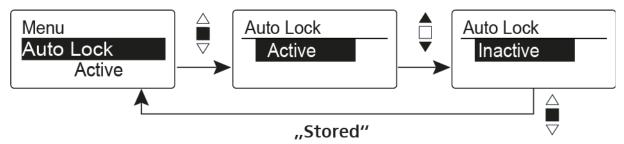
This lock prevents the wireless microphone from being unintentionally switched off and also prevents any unintentional changes to the transmitter's configuration. In the current standard display, the lock icon shows whether the lock-off function is currently switched on.
