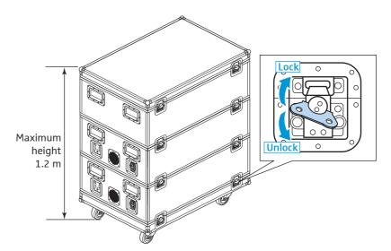
To secure the transport and charging case against inadvertent rolling:
