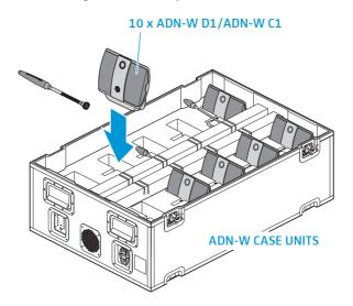
To safely store away the microphones and to insert the goosenecks into the cutouts of the padded compartments:
