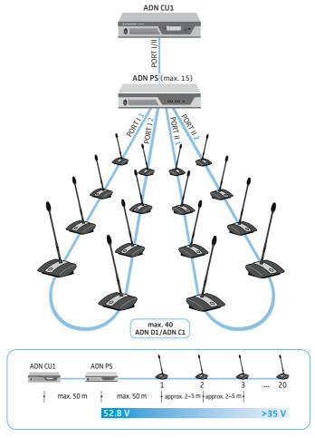
When connecting the conference units to an ADN PS power supply, you can mix different cable topologies (simple cabling with cable strings or redundant ring topology).
