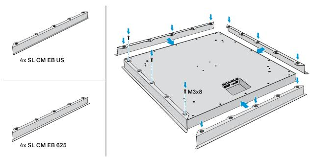
▷ Attach the angle brackets to the TeamConnect Ceiling 2 as shown in the figure.
