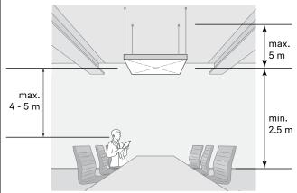
The recommended maximum distance from the speaker to the TeamConnect Ceiling 2 is 4 to 5 m.
