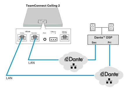
Variant 3: output digital audio signals from multiple ceiling microphones connected in series to one Dante™ network
