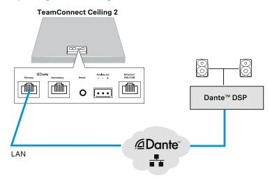
Variant 2: output redundant audio signals to two separate Dante™ networks
