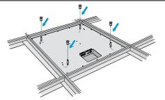
A: secured with SL CM SK suspension kit
