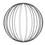
Generally the best way to pick up sound. Microphone position has practically no effect on how/what sound is picked up. Due to possibility of feedback creation, omnidirectional microphones are not recommended to be used in sensitive environment with a lot of reflection - rooms with loudspeaker installations, glass walls etc
