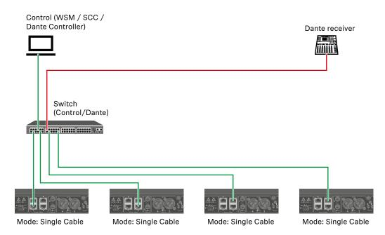
The cable can be connected to socket I, II, III or IV.
