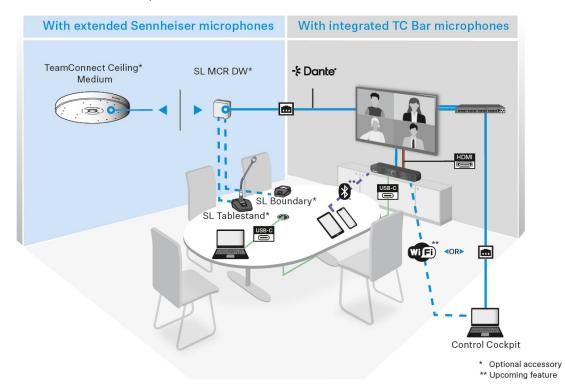
The TC Bar can be integrated into any existing or new network. Different network modes are available, which can be configured for the TC Bar in the Sennheiser Control Cockpit software.
