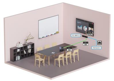
To transmit the incoming video signal from the remote station, the TC Bar can be connected directly to a display via the HDMI cable supplied.
