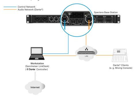
Inside this setup one workstation is used for all client software applications (Sennheiser LinkDesk, Spectera WebUI, Dante® Controller). Either two separated wired network interface are used for control and audio (Dante®) or one interface gets shared. Please be aware that in such setups (typically) no DHCP service is activated. Use either manual IP settings or ZeroConf configuration.
