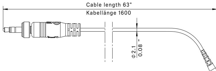
Cable with 3-pin special connector
